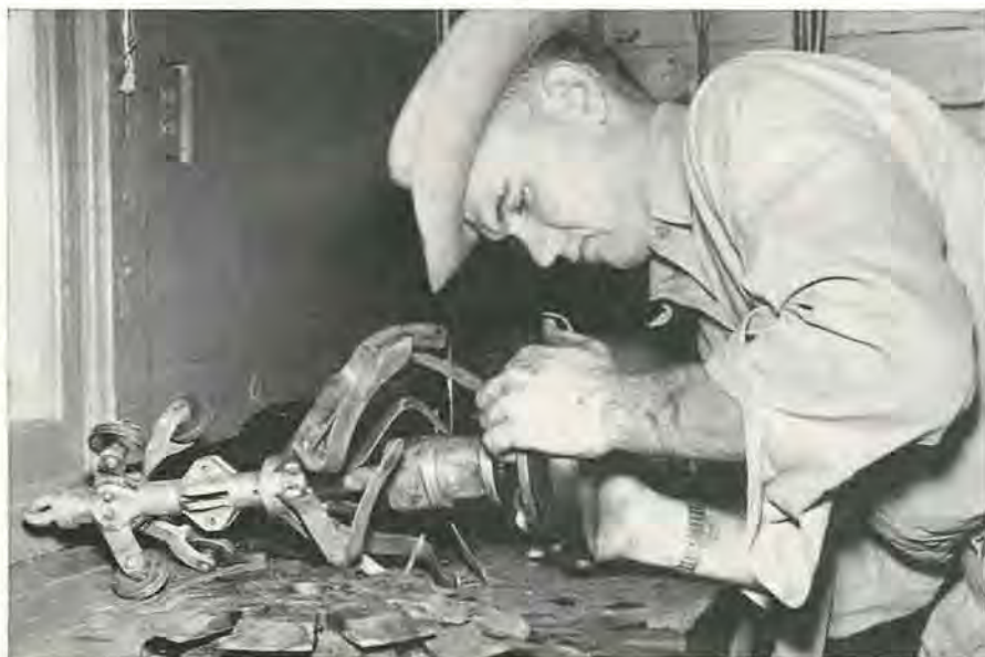
J. D. Andersen, pipeliner, replaces synthetic rubber discs on a scraper-type go-devil at the Baytown Station. Note the notched rubber discs in the foreground which were designed by O. C. Mudd, retired SPL engineer.
